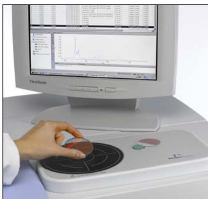
Figure 3. Samples are simply placed on the URA sample platform.
