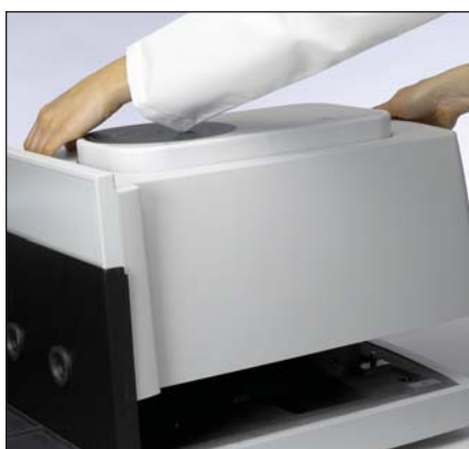
Figure 4. The URA sampling module can be simply interchanged depending on sampling need.
