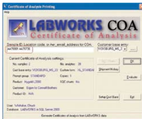
Figure 3. LABWORKS COA program provides a real life solution when combining Storage Tank data with key parameter data on shipment samples by using multiple samples to produce the COA.
