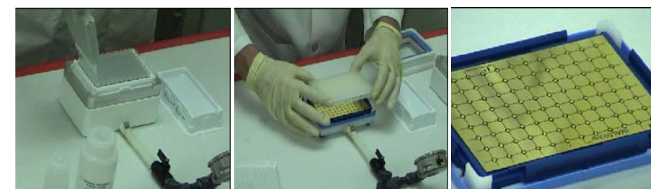
Figure 3. Processing of 96 samples using ProXPRESSION Biomarker HT Kits. These kits fractionate/enrich carrier-protein bound protein fragments (processing may be automated on liquid handlers).
