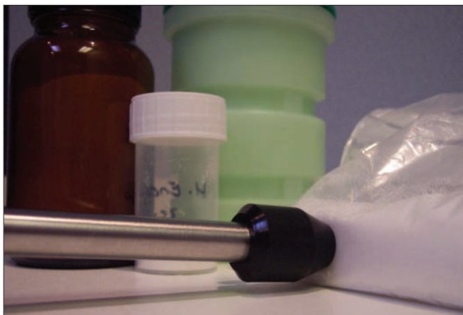
Figure 1. Raman spectra can be collected by holding the Raman probe against the sample container.
