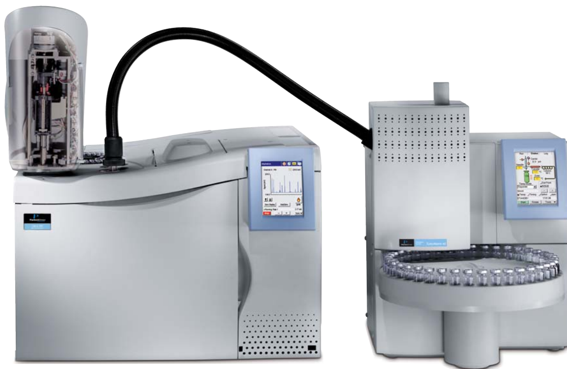
Figure 1. TurboMatrix Automated Headspace Sampler (right) with the Clarus 500 Gas Chromatograph (left).
