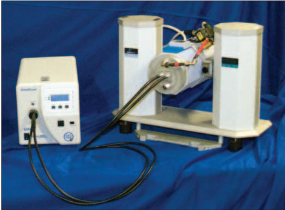
Figure 6. DMA 8000 with special fixture to allow the study of photo-curing systems.
