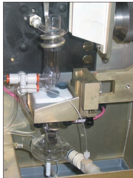
Optima 7300V interior torch view. Note the simple argon quick-disconnect and easy access to the spray chamber and nebulizer.
