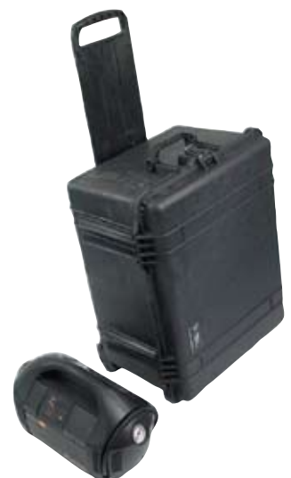
Figure 6. Raman IdentiCheck is packed into a robust case with retractable handle for transportation.
