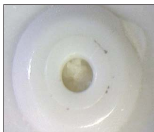
Figure 1. Visible image (x4 objective) of the blockage taken using the camera of the RamanMicro 200.
