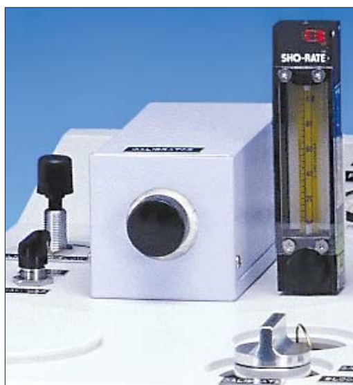
Figure 8. Permeation-tube calibration chamber system.
