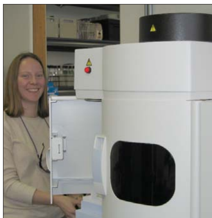
Figure 3. Jacynl Darlow works on a PerkinElmer Optima 5300DV ICP-OES that is used in the analysis of metals in feed samples.
